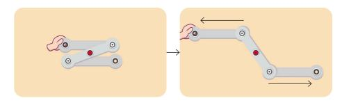
Toolboxes and scissor lifts use linkage mechanisms.
