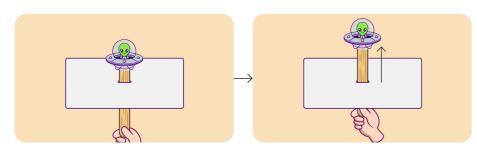
Door bolts and drawers use slider mechanisms.
