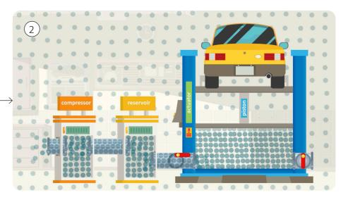
Air is sucked from the atmosphere and squashed in a compressor. The compressed air is stored under high pressure in a reservoir. When the in valve between the reservoir and the actuator is closed, air cannot move out of the reservoir and the piston remains down.
